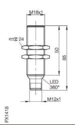
A flush mounted inductive proximity switch from Balluff's Economical Global proximity switch range featuring extended sensing range. M12 connection.
