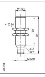
A flush mounted inductive proximity switch from Balluff's Economical Global proximity switch range. M12 connection.
