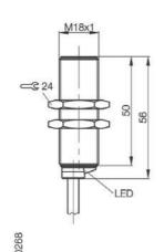
A flush mounted inductive proximity switch from Balluff's Economical Global proximity switch range featuring extended sensing range. Prewired cable
