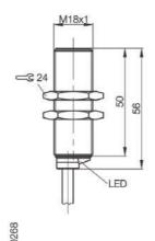
A flush mounted inductive proximity switch from Balluff's Economical Global proximity switch range. Prewired cable.
