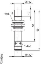
A non flush mounted inductive proximity switch which is PTFE coated and consequently immune from weld splatter. This model also features multimetal technology which allows you to sense other metals such as aluminium or copper without a reduction in sensing distance.
