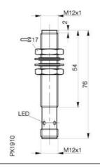
A stainless steel faced flush mounted inductive proximity switch from Balluff's Economical Global proximity switch range.
