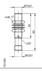
A quasi flush mounted inductive proximity switch from Balluff's Economical Global Tripleprox switch range offering 3 times switching
