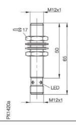
A flush mounted inductive proximity switch which is PTFE coated and consequently immune from weld splatter. This model also features multimetal technology which allows you to sense other metals such as aluminium or copper without a reduction in sensing distance.
