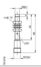
A non flush mounted inductive proximity switch from Balluff's Economical Glogal Tripleprox switch range offering 3 times switching range and M12 connection.
