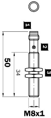
A flush mounted inductive proximity sensor designed to sense ferrous and non-ferrous metals. 3 wire DC operation, featuring short circuit and reverse polarity protection. Also available with extended range, non flush, short body, NPN and N/C please enquire.
