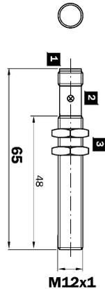
A flush mounted inductive proximity sensor designed to sense ferrous and non-ferrous metals. 3 wire DC operation, featuring short circuit and reverse polarity protection. Also available with extended range, non flush, short body, NPN and N/C please enquire.
