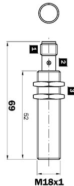
A flush mounted inductive proximity sensor designed to sense ferrous and non-ferrous metals. 3 wire DC operation, featuring short circuit and reverse polarity protection. Also available with extended range, non flush, short body, NPN and N/C please enquire.
