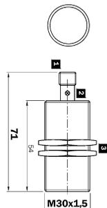
A flush mounted inductive proximity sensor designed to sense ferrous and non-ferrous metals. 3 wire DC operation, featuring short circuit and reverse polarity protection. Also available with extended range, non flush, short body, NPN and N/C please enquire.
