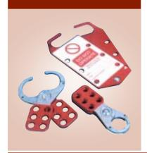
Simple to use lockout hasp allowing multiple key lockout of a single energy source (electrical switchgear, gate valves etc). Manufactured from high tensile steel and plated to resist chemicals and rust. Padlock section covered in thick vinyl to resist wear. Each lockout accepts up to 6 padlocks with up to 9.5mm diameter shackles. Can be used with Prolock padlocks to integrate into a complete interlock system.
