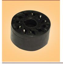
Pcb mounting sockets suitable for 8 and 11 pin relays, picture of 11 pin shown. Rated to 10A at 250VAC.
