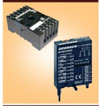
DIN rail mounting IP20 sockets for 11 pin relays. The multifunction version is designed to accept a timer module. The multifunction timer provides a wide variety of timing functions from 0.05 S to 240 hours such as delay on, delay off, single hot, flashing and so on. Its supply voltage range is 24 to 240V ac or dc.
