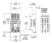
A DIN rail, snap-mount socket with screw terminations and is designed to accept KU series and RM series relays with 4.75mm terminals. Constructed with a spring loaded latch to allow quick installation or removal. This socket is suitable for single, double & three pole relays.
