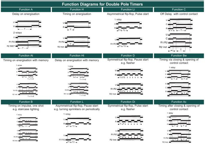
Note: The above timing charts show outputs for single & double pole models, ignore R2 for single pole models. Pin-outs may vary dependant on the style of timer
