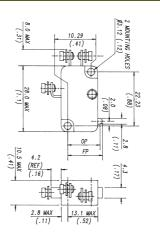
A high temperature V3 miniature microswitch with a maximum continuous working temperature of 240°C. Available with single pole changeover silver contacts and screw terminals.
