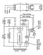
A range of four different auxiliary actuators for V3 style switches comprising of standard plain lever, standard lever with a free running roller, short plain flexing leaf lever or short flexing leaf with roller. All are supplied with frame to fit one switch, an insulating sheet and two M3 x  $25 \mathrm{mm}$  screws with washers and nuts. Use the screws both to mount the frame to the switch and to mount the complete assembly to the application. Suitable for plunger actuated V3 style switches.
