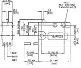
An industry standard V3 miniature microswitch pre-wired and sealed to IP67. Switches are supplied complete with 0.5m PVC cable. Available with a variety of integral levers.
