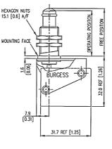
An hole mounted standard V3 miniature microswitch pre-wired and sealed to IP67. Installation via mild steel threaded sleeve provides convenient method of adjusting position. Available with plain plunger or roller actuator. Switches are supplied complete with 0.5m PVC cable.
