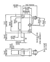
A single pole miniature microswitch with normally closed positive break contacts which are forced open to 3mm (min gap), even in the event of welding. Featuring a roller lever actuator (11.7mm) and 6.3mm 'push-on'
