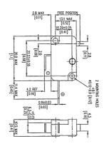
A single pole miniature microswitch with normally closed positive break contacts which are forced open to 3mm (min gap), even in the event of welding. Featuring standard plunger actuator and 6.3mm 'push-on' terminals.
