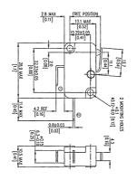
A single pole miniature microswitch with normally closed positive break contacts which are forced open to 3mm (min gap), even in the event of welding. Featuring a standard (13.7mm) or extended (26.2mm) plain levers and 6.3mm 'push-on' terminals.
