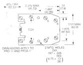
Heavy duty power relay with DPCO contacts capable of switching 25A. Suitable for industrial control applications. Durable, robust mounting base with screw terminal connections.
