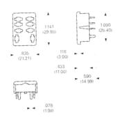
DIN and PCB mounted sockets for use with K10 style relays. IP20 finger protection with M3.5 captive terminal screws on the DIN sockets. PCB sockets are manufactured with "floating" loose terminals which permits them to align with holes in the circuit board and with the relay terminals. Hold down springs for relay retention are also available, please order separately.
