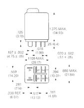
A plug-in general purpose DPCO miniature relay with 15A capacity. Compact in size it is ideal for installation in small equipment.
