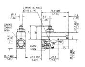
A single pole changeover microswitch housed in aluminium offering high reliability and long life in harsh industrial environments. Insert switch attached to lid provides quick and efficient installation. Available with a standard plunger actuator.
