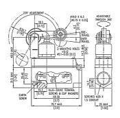
A single pole changeover microswitch housed in aluminium offering high reliability and long life in harsh industrial environments. Insert switch attached to lid provides quick and efficient installation. Available with a cowl protected roller lever adjustable through 360° horizontally and 235° vertically
