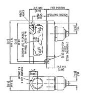
A single pole changeover microswitch housed in aluminium offering high reliability and long life in harsh industrial environments. Insert switch attached to lid provides quick and efficient installation. Available with a cowled standard plunger actuator offering IP67 protection
