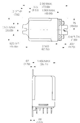
A flange mounted SPCO enclosed power relay with a 30 Amp switching capability.
