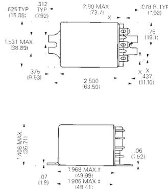
A flange mounted DPCO enclosed relay with a special insulation barrier to gain approval to VDE 0453. It has 8mm spacing between contacts and coil to satisfy needs for insulation between low voltage circuits and power circuits.
