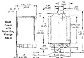
A flange mounted DPCO enclosed power relay with a 20 Amp switching capability.
