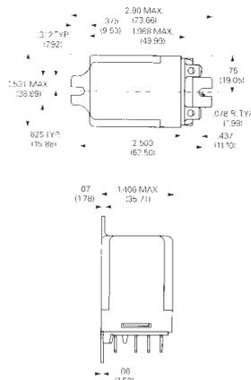
A flange mounted DPCO enclosed power relay with a 20 Amp switching capability.
